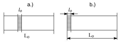
Fig. 9 Fabric sample as the serial connection of a single breaking E-bundle and an elastic part
