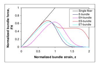
Fig. 3 Expected value of typical normalized force-strain curves of the FBCs
