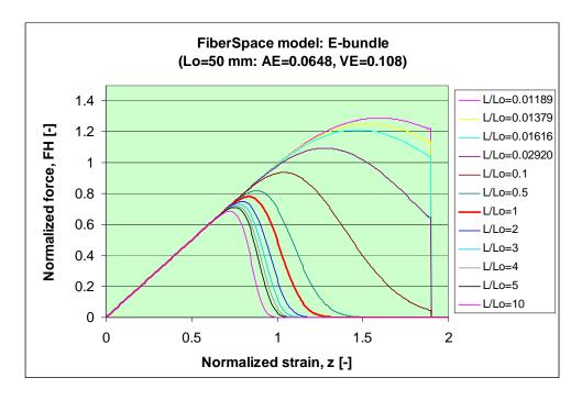
Fig. 10 Normalized expected force-strain curves of E-bundles with different relative lengths  $(L/L_o)$
