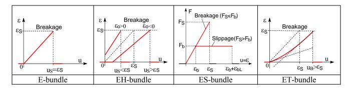
Fig. 2 Relationship between the strains of single fibers and FBCs
