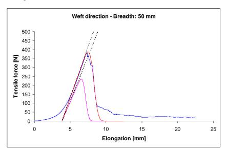
Fig. 12 Measured and averaged force-elongation curve (blue line), shifted E-bundle curve (lilac line), and the transformed model curve (red line) for samples cut out of weft direction
