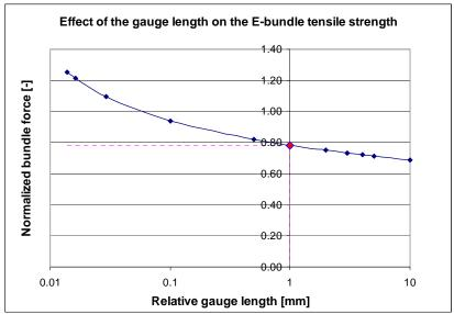
Fig. 11 Peak values of E-bundles versus relative yarn length in logarithmic scale Figs. 12 and 13 show the measured and averaged force-elongation curves (blue lines) and the steepest tangents.
