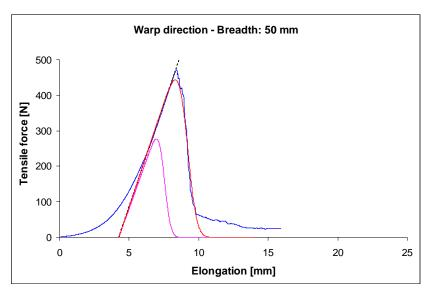
Fig. 13 Measured and averaged force-elongation curve (blue line), shifted E-bundle curve (lilac line), and the transformed model curve (red line) for samples cut out of warp direction
