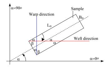
Fig. 6 Disposition of a sample to the main structural directions of the fabric
