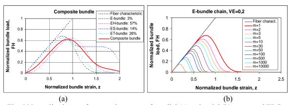
Fig. 5 Normalized mean force-strain curves of parallel (a) and serial (b) connected FBCs
